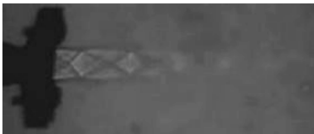
Fig. 21 Shadowgraph picture for uncontrolled jet at NPR 4.
