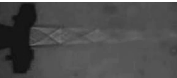
Fig. 23 Shadowgraph picture for uncontrolled jet at NPR 5.74.
